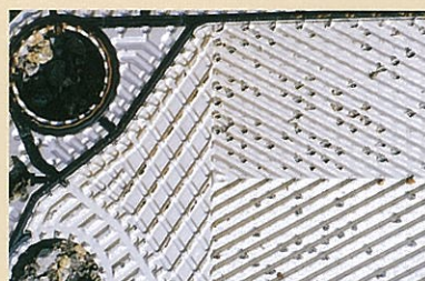
(right) 3 months after chemical treatment Hard white encrustation of hard scale (Can be removed by chemical cleaning only.)
