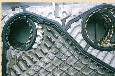
(left) 10 months after installation of SUPRION Soft sludge (Readily removed by brush cleaning)
